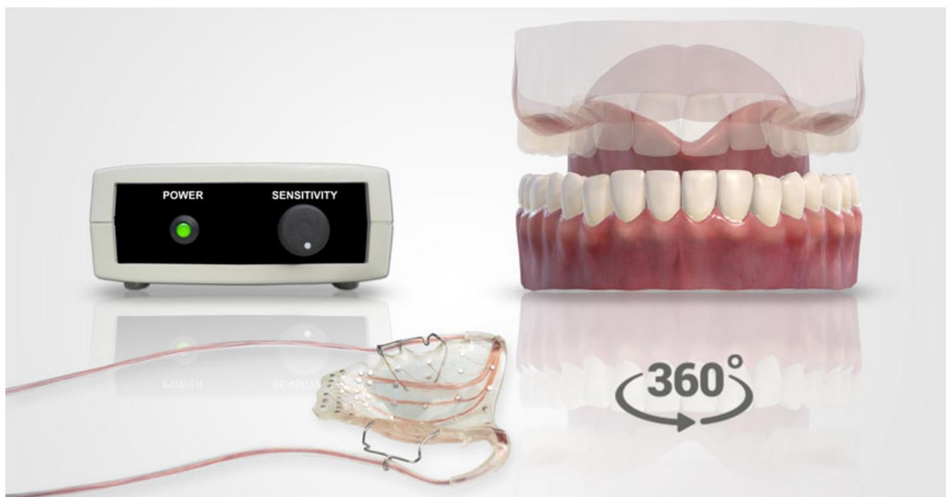
3D Electropalatography (3D EPG) uses state-of-the-art computer animation and 3D modelling techniques to illustrate where the tongue touches the hard-palate during speech. The 3D model, which can be rotated 360°, provides direct articulatory information in real-time.
