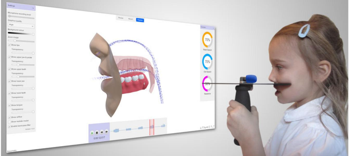
The Nasality Microphone is a handheld nasometry unit that detects the nasality in speech production. It uses a lightweight acoustic separator that is fitted with highly directional nasal and oral microphones. The portable design and USB compatibility makes the Nasality Microphone ideal for clinical or home-based speech therapy.
